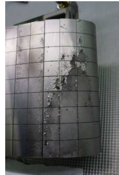
Erosion of JET Iter-like Wall
